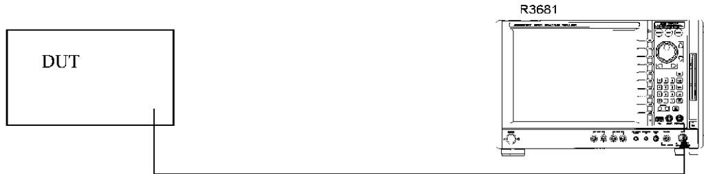
Figure 4-15 Connection Diagram for the Modulation Analysis that Uses the Multi Frame Mode
