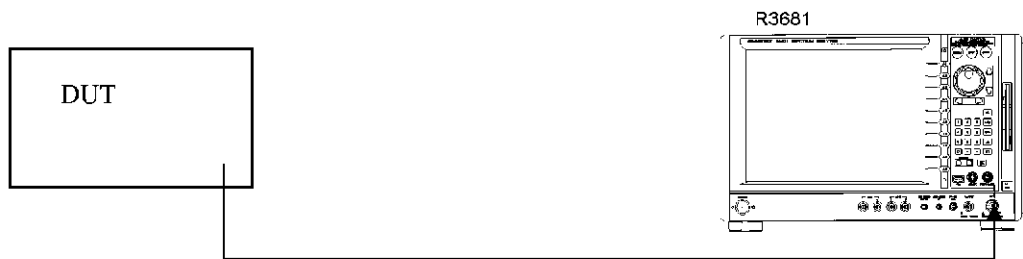
Figure 4-20 Connection Diagram for the Modulation Analysis that Uses the Multi Frame Mode
