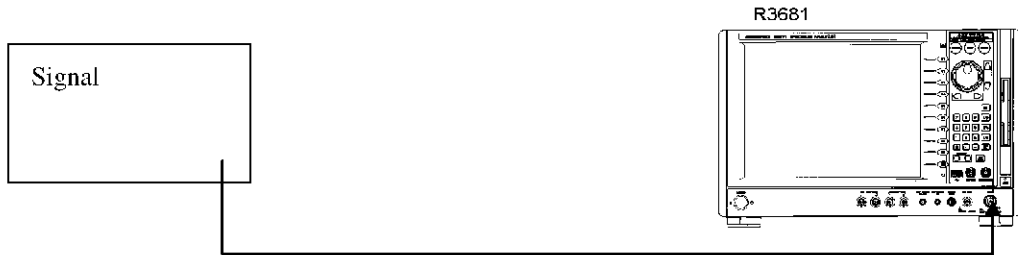
Figure 4-7 Connection Diagram for the Modulation Analysis that Uses the Single Frame Mode
